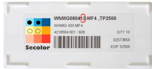
Figure 11: The nose radius can be found as the last two figures in the identification number for the insert geometry. This can be found on the underside of the insert box.
